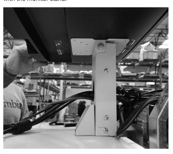
9) Using the 4 Sems Pan Head screws and the provided screwdriver, secure the monitor to the monitor stand.
