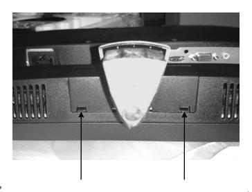
3) Remove the two screws on the stand.
