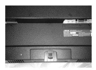
6) Remove the 4 Vesa plugs on the back of the monitor. These can easily be popped out with your finger. (Removed plugs shown below)
