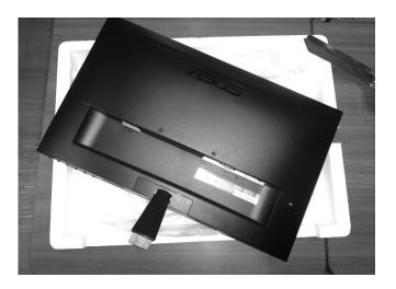
2) Remove the stand cover by pushing the two clips in and pulling out. Keep to the side for now.
