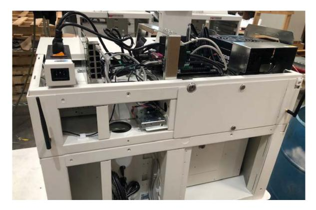
9. Find the barrel jack connector inside the bin module. Then route it up through the body holes and connect it to the power distribution block.
