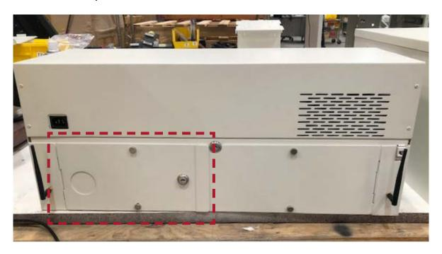
6. Using a 5/16 wrench remove the nuts from the small plate and remove plate.
