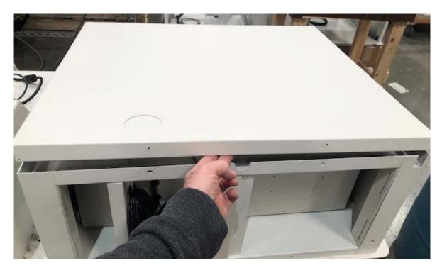
3. Using a 5/16" nut driver or socket, remove the 4 nuts from the plate, then remove the plate.
