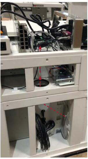
12. Re-install the top on the computer module, replace all panels on the back of the machine including all thumbscrews and lock all panels.
