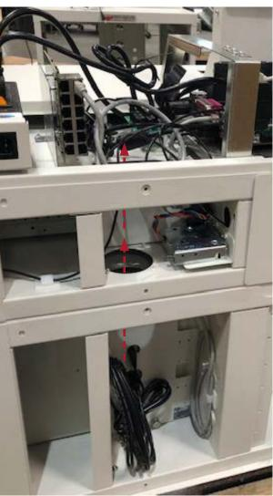
10. Find the usb cable in the bin module, route up through the body holes and connect to an open usb port.
