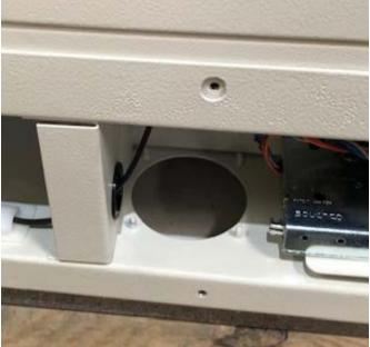
7. Stack the computer module on top of the bin module and install the connecting plates on both sides.
