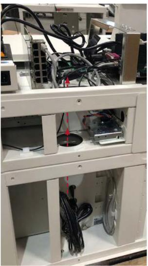
11. Find the CAT5 Ethernet cable in the bin module, route up through the body holes and connect to the StatSafe main board in the top CAT5 port on the front of the main board pictured below.
