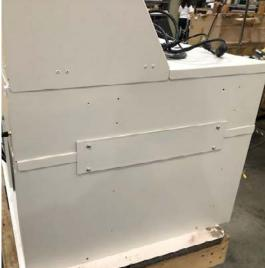
8. Remove the top cover from the computer module by unlocking the top lock, sliding the cover backwards to the rear and then lifting up.
